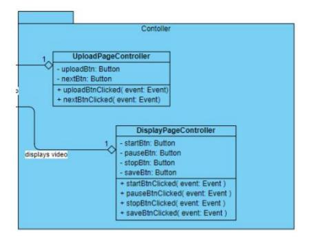
This package is responsible for providing the user with a way to interact with the application. There are various button objects that provide different functionality for the UI.
