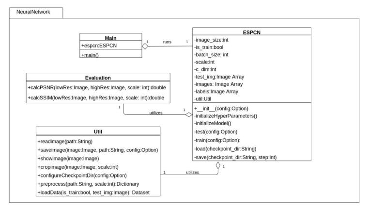
To train models, we planned to apply transfer learning on ESPCN, an OpenCV model that can do real time video upscaling. This package includes the classes which are used for training, evaluating, and testing the model.
