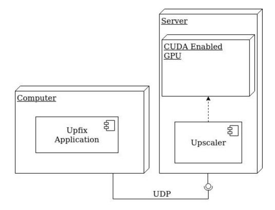
The user must have a CUDA enabled GPU to use our desktop application. Like in the web application, the GPU will be used to speed up inference and video rendering time.
